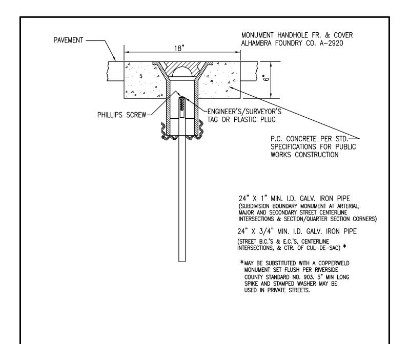
MONUMENT SHALL BE FURNISHED AND SET BY A LICENSED SURVEYOR OR REGISTERED CIVIL ENGINEER. MONUMENT SHALL CONSIST OF SURVEYOR'S OR ENGINEER'S TAG SECURED WITH A ROUND HEAD PHILLIPS SCREW SET TO TRUE POSITION IN TOP OF CEMENT MORTAR CORE IN GALVANIZED IRON PIPE OR A STAMPED PLASTIC PLUG.
